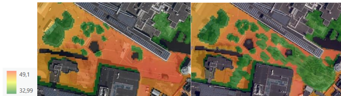
Figure 3 Digital Twin: temperature at Campus B before (left) and after (right) planting trees
